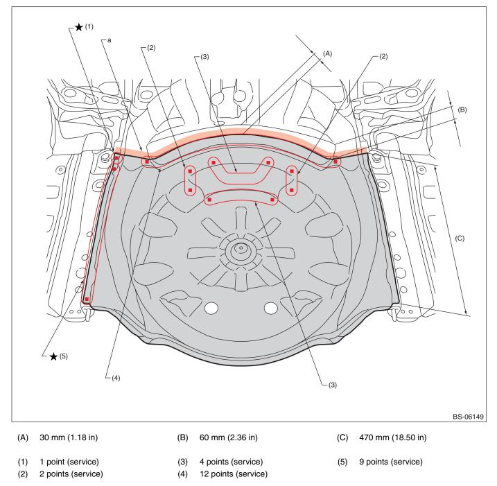
Note: Apply a sealing agent to the floor pan panel fitting parts of part "a".
